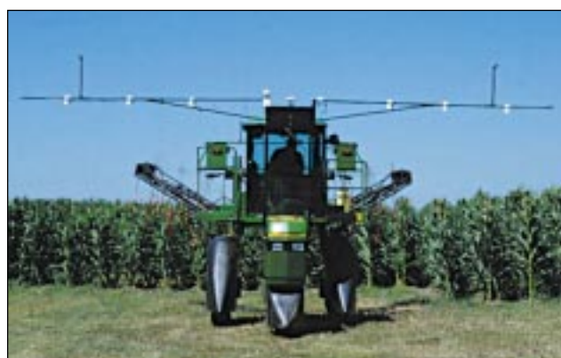
Figure 3. High-clearance applicator equipped for on-the-go sensing of crop N status and variable-rate N application (Photo provided by USDA-ARS, Lincoln, Nebraska).
