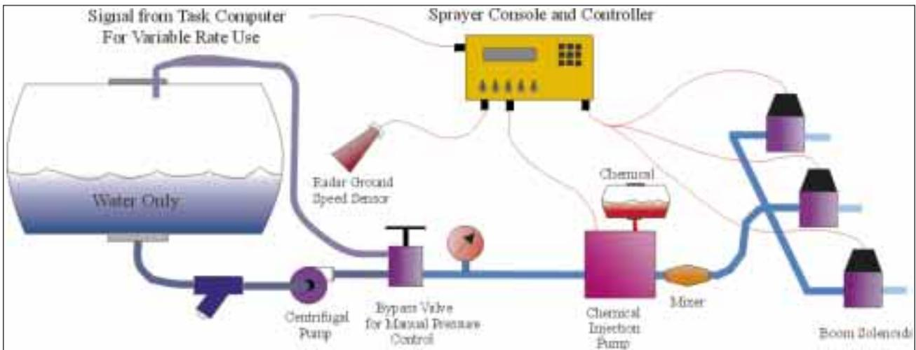
**Figure 2.** A direct chemical injection system. Water flow rate is set separately by adjusting pressure. If the controller will accept an RS 232 rate command, a task computer can be used to apply variable rates.
