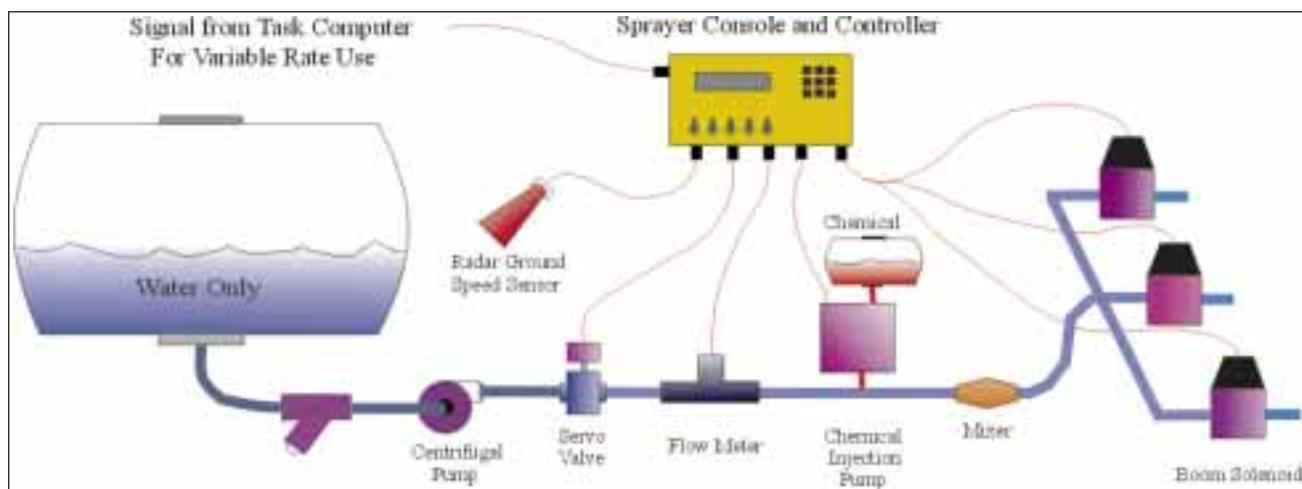
**Figure 3. A chemical injection system with carrier control. The system increases or decreases both chemical flow rate and water flow rate to match ground speed variations. Controllers that accept external inputs of rate commands can do variable rate application.**
