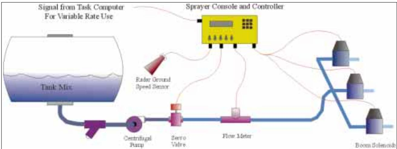
**Figure 1.** A simple tank mix system that varies flow rates to match ground speed variation. If the controller will accept an RS 232 input for a rate command from a task computer this system can do variable rate application.
