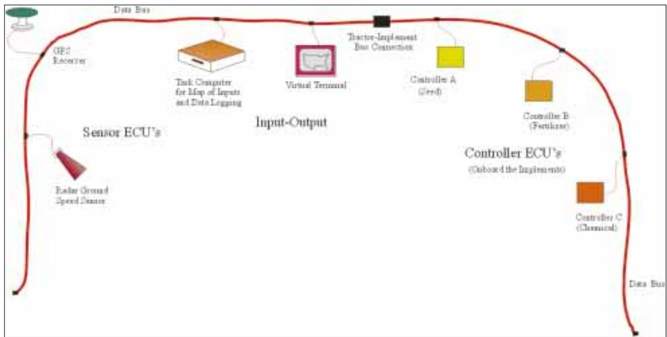
**Figure 2. The simplified wiring of a CAN and the J1939 network protocol. All messages from devices on the network are available to other devices. Maps developed on a desktop computer can be loaded into the task computer via a PCMCIA card.**
