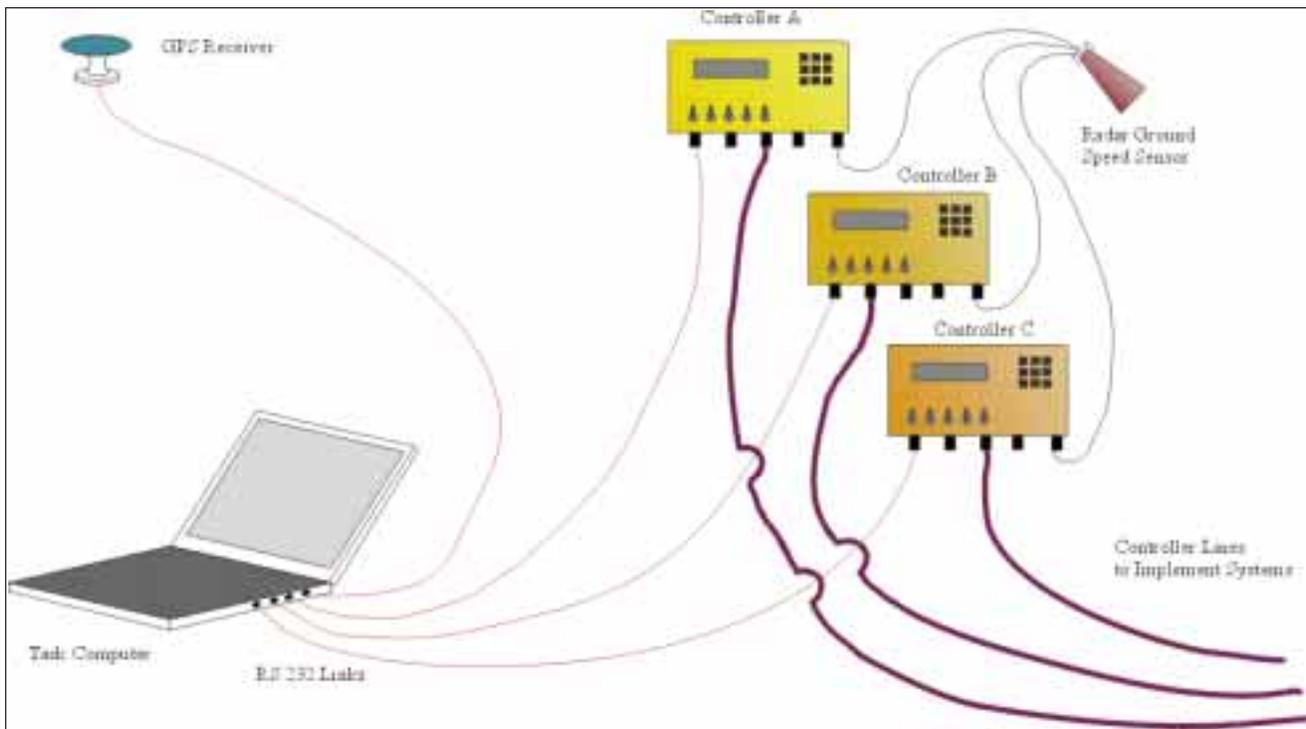
Figure 1. Wiring concept for a three-input variable system. The task computer requires four RS 232 serial ports to communicate.
