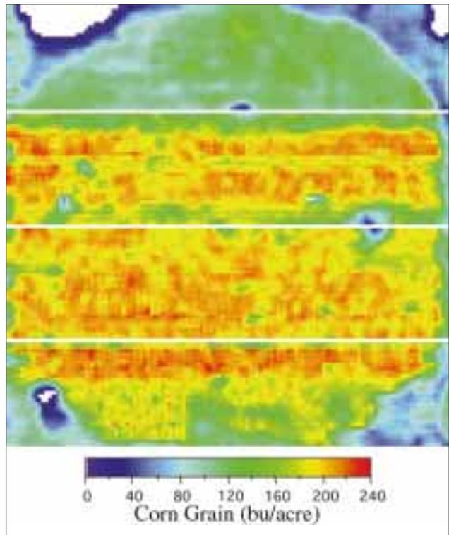
**Figure 2.** Yield map generated with yield monitor data and differentially-corrected GPS data.
