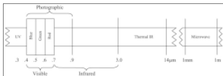
Figure 1. The electromagnetic spectrum.
