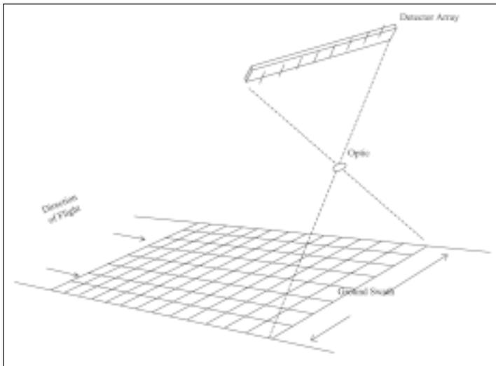
**Figure 5. A linear array pushbroom multispectral scanner.**
