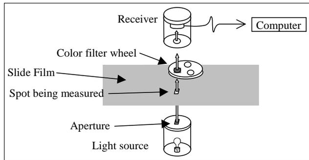
**Figure 3. The process and components of making a densitometer measurement.**
