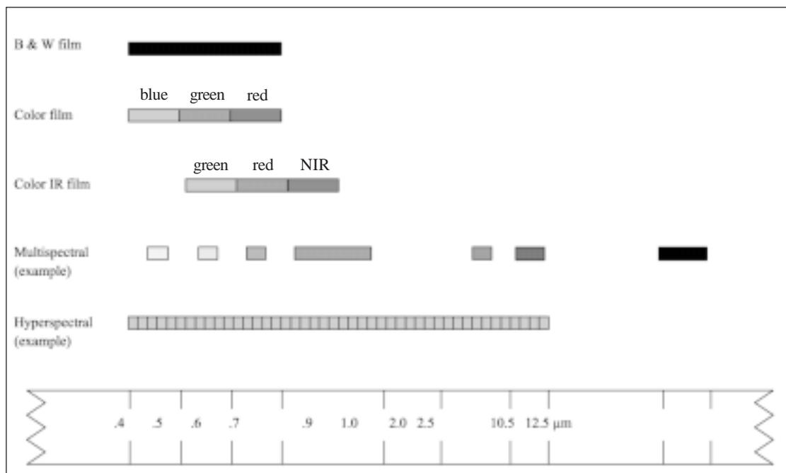
**Figure 4. A graphical representation of the regions in which photographic and multispectral scanners sense.**
