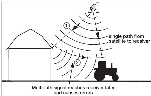
**Figure 2. GPS signals can sometimes “bounce” off of objects in their path and cause the signal to reach the receiver on a different path. This is called multipath error.** (Deere & Company ©)
