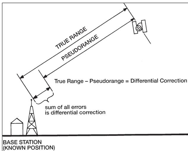
**Figure 3.** A stationary receiver (base station) measures its distance from each satellite (pseudorange) and then calculates the error pseudorange minus true distance). This error is called the differential correction. (Deere & Company ©)
