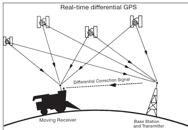
**Figure 4.** In real-time DGPS, the stationary receiver transmits the differential correction to the moving receiver via another radio signal. (Deere & Company ©)
