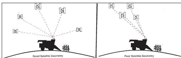
**Figure 1. Good satellite geometry (widely and evenly-spaced satellites) yields more accurate GPS position estimates than poor satellite geometry.** (Deere & Company ©)
