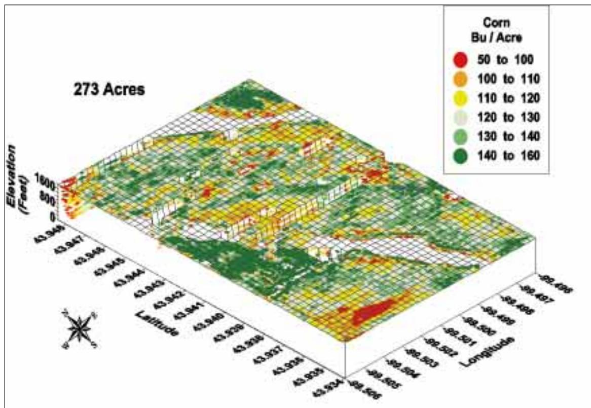
Figure 2. Your yield map superimposed on a topography map generated from real-time kinematic code-phase DGPS.
