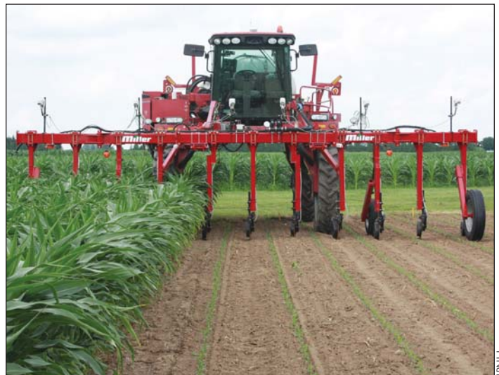
Mid-row coulter-style liquid fertilizer bander for corn.
