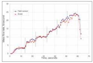
Figure 5a. Response to increasing yield at a constant ground speed in the field.
