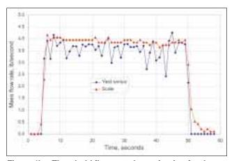
Figure 4b. Threshold flow rate determination for the yield sensor.
