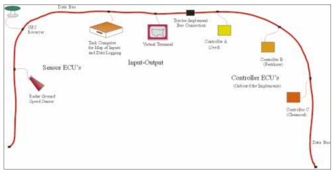
Figure 2. The simplified wiring of a CAN and the J1939 network protocol. All messages from devices on the network are available to other devices. Maps developed on a desktop computer can be loaded into the task computer via a PCMCIA card.
