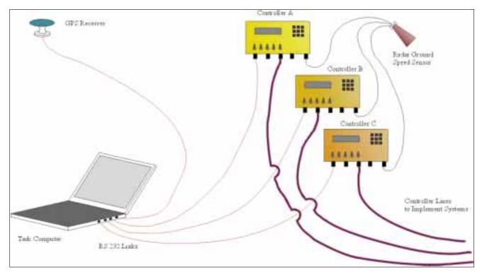
Figure 1. Wiring concept for a three-input variable system. The task computer requires four RS 232 serial ports to communicate.
