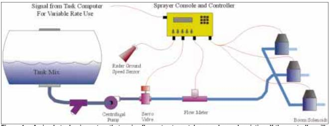
Figure 1. A simple tank mix system that varies flow rates to match ground speed variation. If the controller will accept an RS 232 input for a rate command from a task computer this system can do variable rate application.
