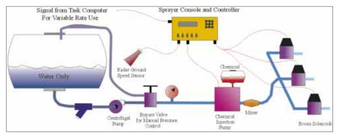
Figure 2. A direct chemical injection system. Water flow rate is set separately by adjusting pressure. If the controller will accept an RS 232 rate command, a task computer can be used to apply variable rates.
