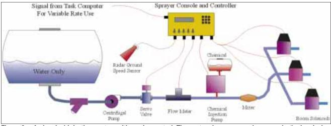
Figure 3. A chemical injection system with carrier control. The system increases or decreases both chemical flow rate and water flow rate to match ground speed variations. Controllers that accept external inputs of rate commands can do variable rate application.
