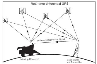
Figure 4. In real-time DGPS, the stationary receiver transmits the differential correction to the moving receiver via another radio signal. (Deere & Company ©)
