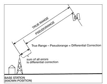
Figure 3. A stationary receiver (base station) measures its distance from each satellite (pseudorange) and then calculates the error pseudorange minus true distance). This error is called the differential correction. (Deere & Company ©)
