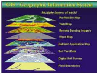
Figure 11. Multiple layers of several data sets are used in a GIS to develop a map of the variability in profit for a field (Rund, 1999).
