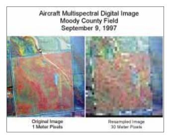
Figure 1. False color imagery of a farm field is represented in two pixel resolutions (1 m versus 30 m pixels). Observable differences in detail between the scenes are obvious from individual trees to drainage definition. Similarities between scenes are seen in the crop vigor (strength of red colors) and northwest-southeast orientation of coloration differences.
