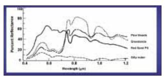
Figure 2. Typical reflectance of four features is plotted across a part of the electromagnetic spectrum from blue light to near infrared light. Note the characteristic "jump" in reflectance between 0.7 and 0.8 µm (where reflective infrared begins) for growing vegetation as well as the differences in curves between grasslands and pine.
