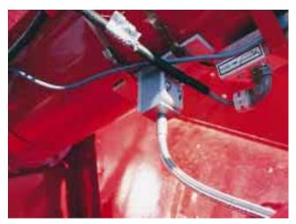
Figure 1. Grain quality monitor mounted to the outlet auger of a combine harvester.
