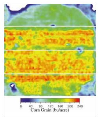
Figure 2. Yield map generated with yield monitor data and differentially-corrected GPS data.
