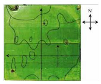
Figure 1. Aerial photo of quarter section illustrating soil boundaries. Strips are laid out perpendicular to maximum soil variation (north-south solid line). In areas where soil properties are uniform, strips can be laid out in either direction (dashed lines).
