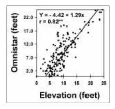
Figure 4. The relationship between elevation measured by laser and elevation measured by a RTK code-phase DGPS.
