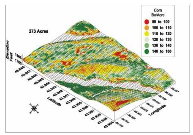
Figure 1. The competitor's yield map superimposed on topography map generated from a real-time kinematic carrier-phase DGPS.
