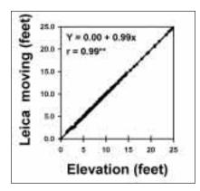
Figure 3. The relationship between elevation measured by laser and elevation measured by a RTK carrier-phase DGPS.
