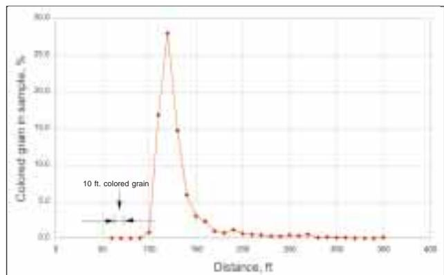
**Figure 1. Colored grain flow through combine.**
