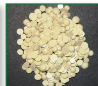
Sulfur pastilles, containing small amounts of clay to enhance dispersion and oxidation
