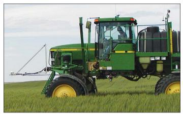
Active crop sensor attached to the front of a liquid N fertilizer applicator.
