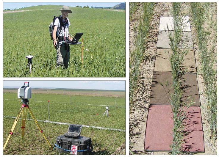
**Dr. Jan Eitel taking remotely sensed measurements** in a field of spring wheat. Scanning green laser equipment is shown measuring early stage crop N status (bottom left). Inserted trays of different colored soils were used to measure the effect of soil background reflectance on vegetation indices used for inseason N management (right).
