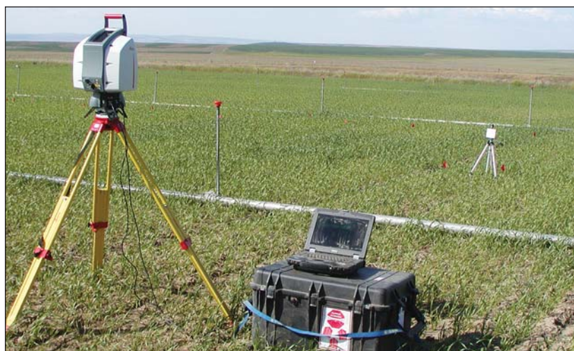
Dr. Jan Eitel taking remotely sensed measurements in a field of spring wheat. Scanning green laser equipment is shown measuring early stage crop N status (bottom left). Inserted trays of different colored soils were used to measure the effect of soil background reflectance on vegetation indices used for in-season N management (right).
