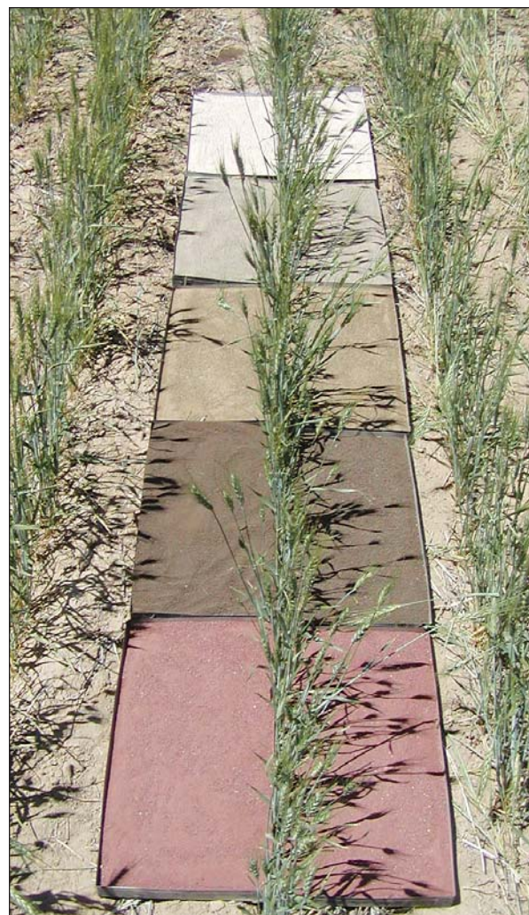
Dr. Jan Eitel taking remotely sensed measurements in a field of spring wheat. Scanning green laser equipment is shown measuring early stage crop N status (bottom left). Inserted trays of different colored soils were used to measure the effect of soil background reflectance on vegetation indices used for in-season N management (right).
