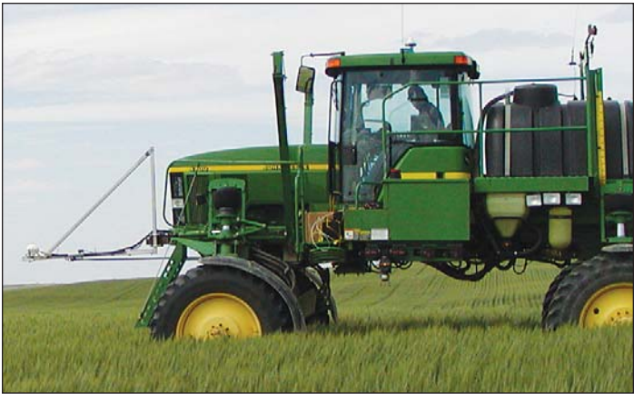
Active crop sensor attached to the front of a liquid N fertilizer applicator.
