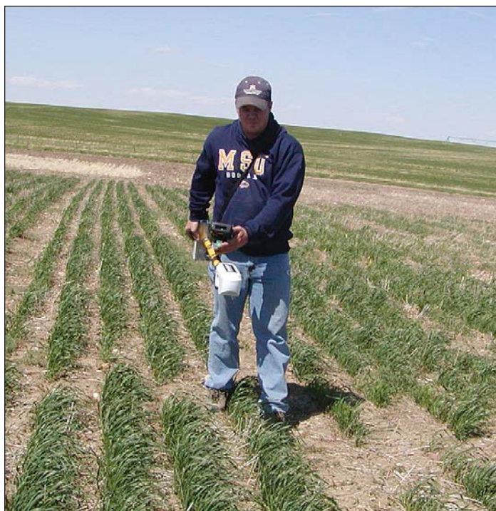
Obtaining spring wheat reflectance measurements (Left: Robin Christiaens, Research Associate using GreenSeeker Sensor, and Right: Jeff Jerome, Research Assistant using Pocket Sensor), Western Triangle Agricultural Research Center, Conrad, MT, Spring 2012.
