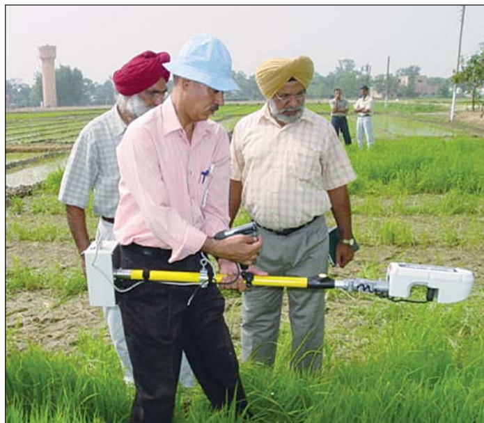
Demonstration of GreenSeeker™ optical sensor technology on-farm with lead author on the left.
