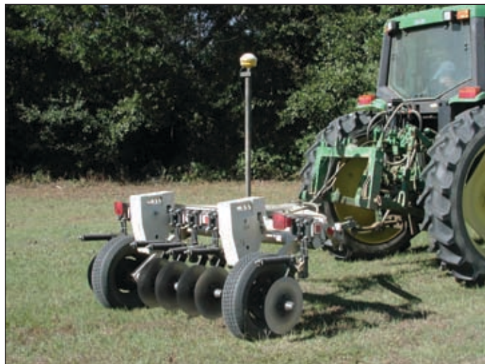
A view of the Veris 3100 soil electrical conductivity equipment.
