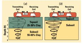
Figure 1. EM-38 principle of operation in soils.
