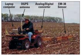
Figure 2. Mobile EM-38 sensor unit is pulled behind a four-wheel ATV, equipped with analog/digital converter, laptop computer, and DGPS antenna.
