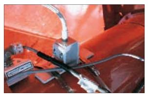
**The sensor** is shown here mounted on a combine during protein and moisture testing.
