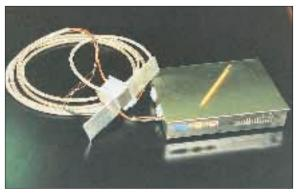
**This sensor** uses multi-spectral optics to measure protein content in wheat during harvest. (Source: Milestone Technologies, Inc.)
