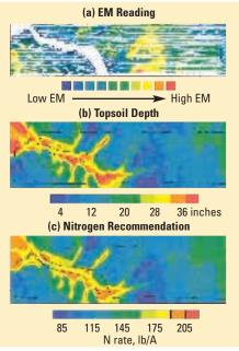
Figure 4. EM-38 soil conductivity, topsoil depth, and N recommended for corn at Centralia, Missouri.
