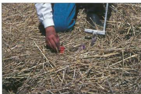
THE PRS probes are buried in the soil.
