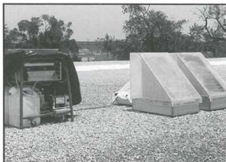
SOLAR REACTORS for studying the \text{TiO}_2 catalyzed degradation of pesticides.
