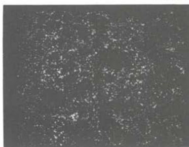
FIGURE 2 —Here is the electron microprobe's visual picture of K, Ca, and Mg in mint stem tissue harvested from soils containing 340 and 40 lb K/A. Note high intensity of white dots in stem from high-K soil, low intensity from low-K soil.
