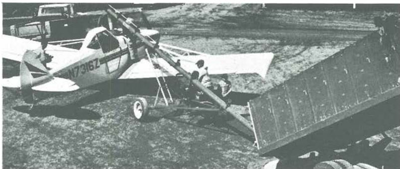
Airplane and the "reload" setup which Mr. Wells uses to seed small grain.
