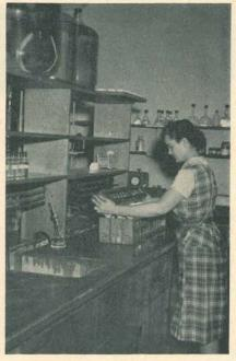
Filtering is one of the steps necessary in testing soils. Here an Oregon State technician works on some samples. Picture courtesy Oregon Agricultural Experiment Station.
