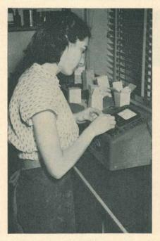
Soil Reaction (pH) is determined on all soil samples that come into a soil testing laboratory. Here an Oregon State technician runs a sample. Picture courtesy Oregon Agricultural Experiment Station.
