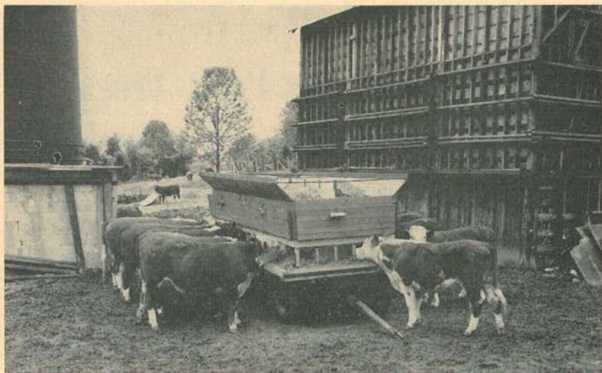
Fig. 1. This self-feeder wagon for use with chopped green feed was built by Robert Barnhardt, Fiddler's Creek Farm, Titusville, New Jersey.
