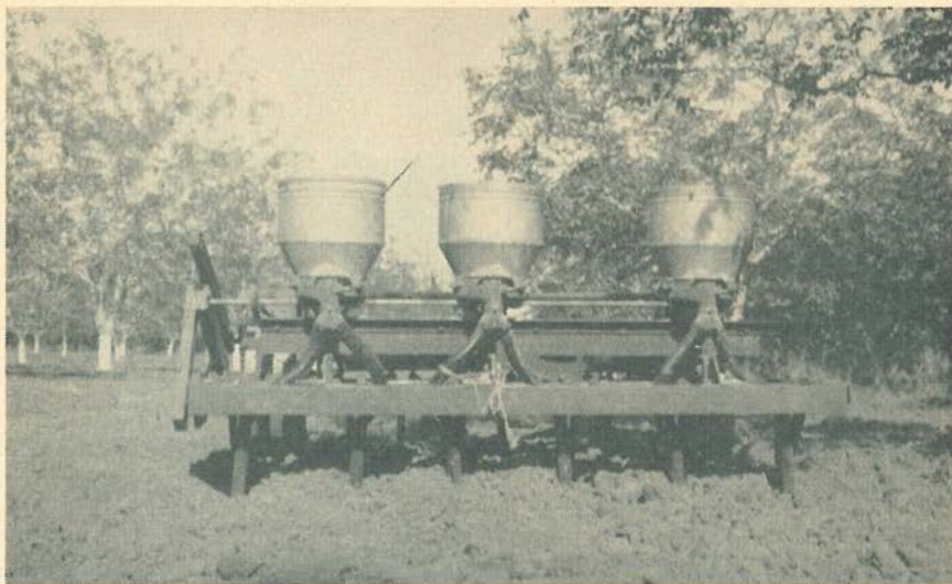
Fig. 4. Drill for deep placement of fertilizer in orchards. The frame is specially built. Fertilizer attachments are standard manufactured equipment.
