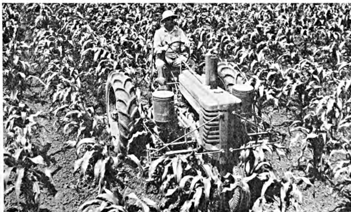
Fig. 2. Sidedressing attachments for all makes of tractors are available. The application of from 125 to 150 lbs. of ammonium nitrate (or its equivalent in other nitrogen fertilizers) is recommended when corn is about knee-high.
