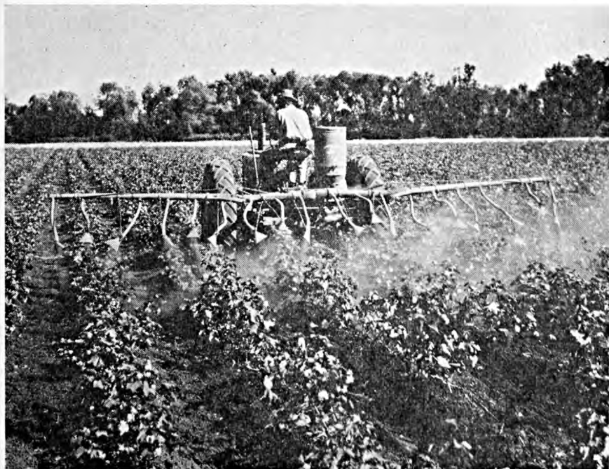
Below: Tractor-mounted equipment can apply insecticides and defoliants to as many as 40 acres of cotton per day.
