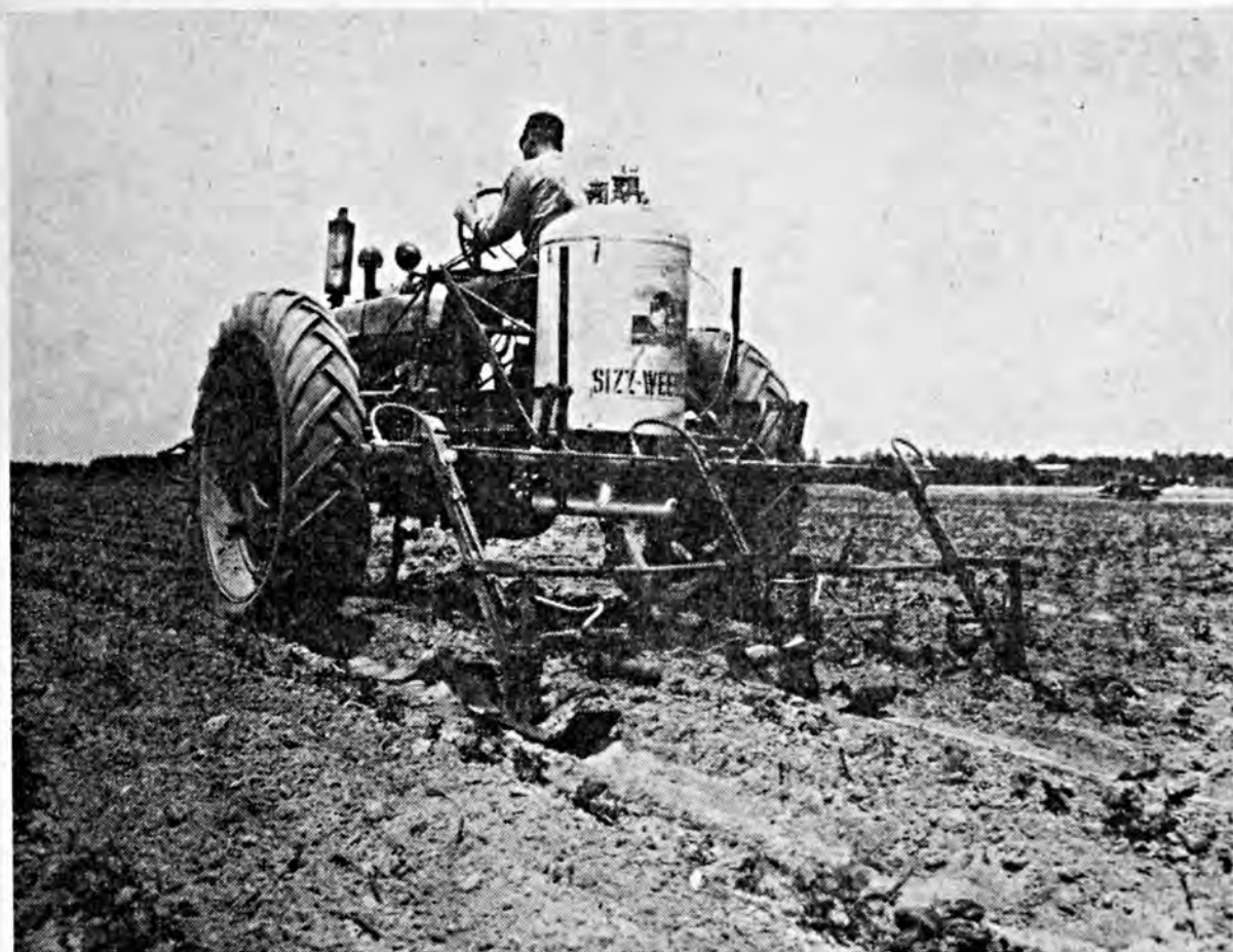
Above: Searing jets of flame from this two-row flame cultivator kill weeds and grass but do not harm cotton.
