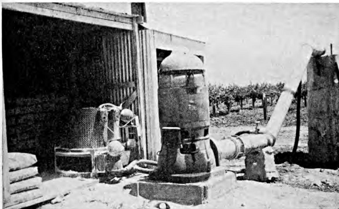
Fig. 8. Permanent installation of gypsum applicator manufactured by the Delano Engineering Co.
