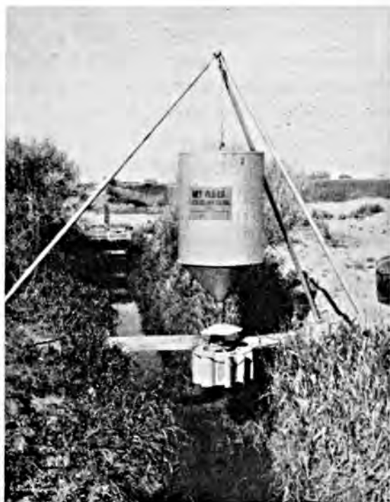
Fig. 3. Dry-Flo Fertilizer Co. Applicator set up over irrigation ditch, prior to turning on water.
