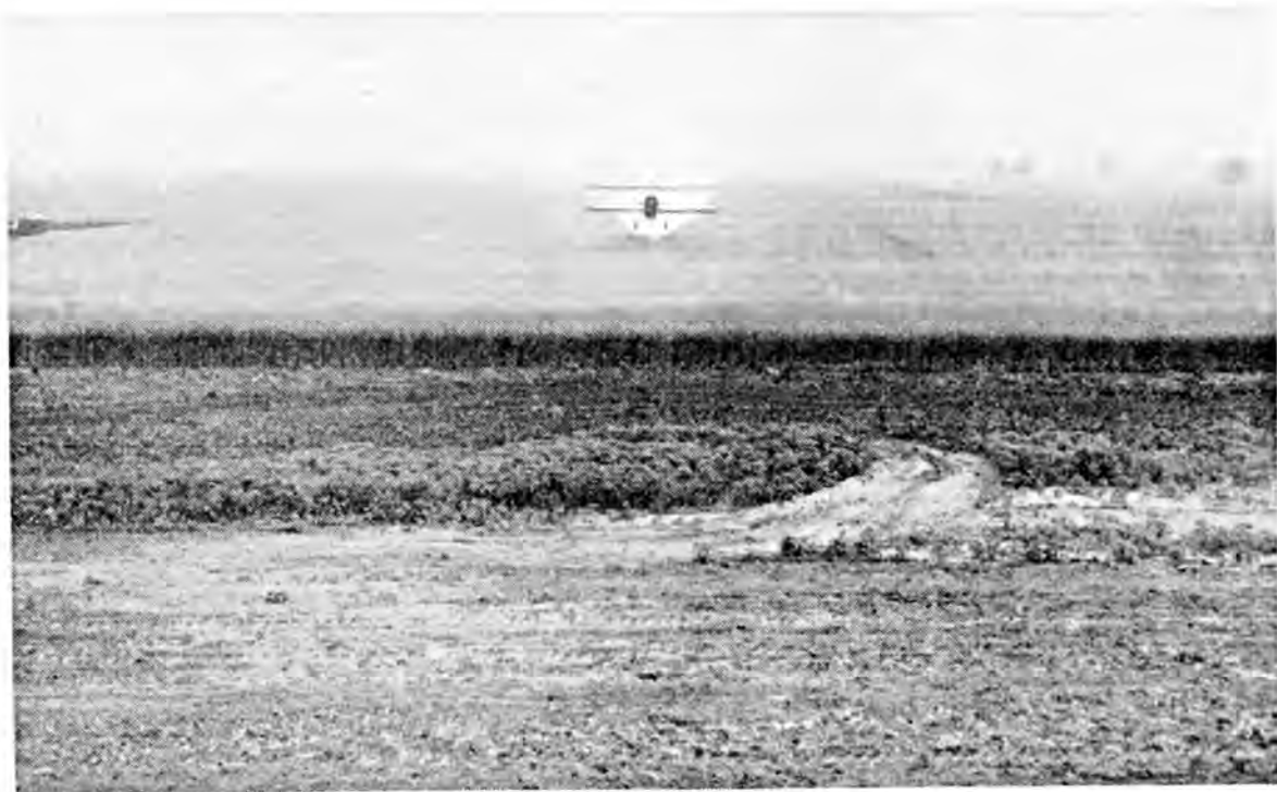
Fig. 5. Twenty pounds of dusting sulfur per acre were applied for the control of black stem rust. The applications were made in the early morning when the air was still and there was dew or moisture on the wheat. The sulfur remained until harvest time in areas where no heavy rains fell.
