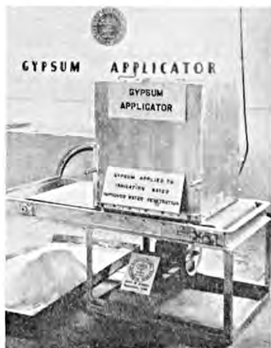
Fig. 2. Gypsum applicator designed by University of California, Agricultural Extension Service, Kern county, California.
