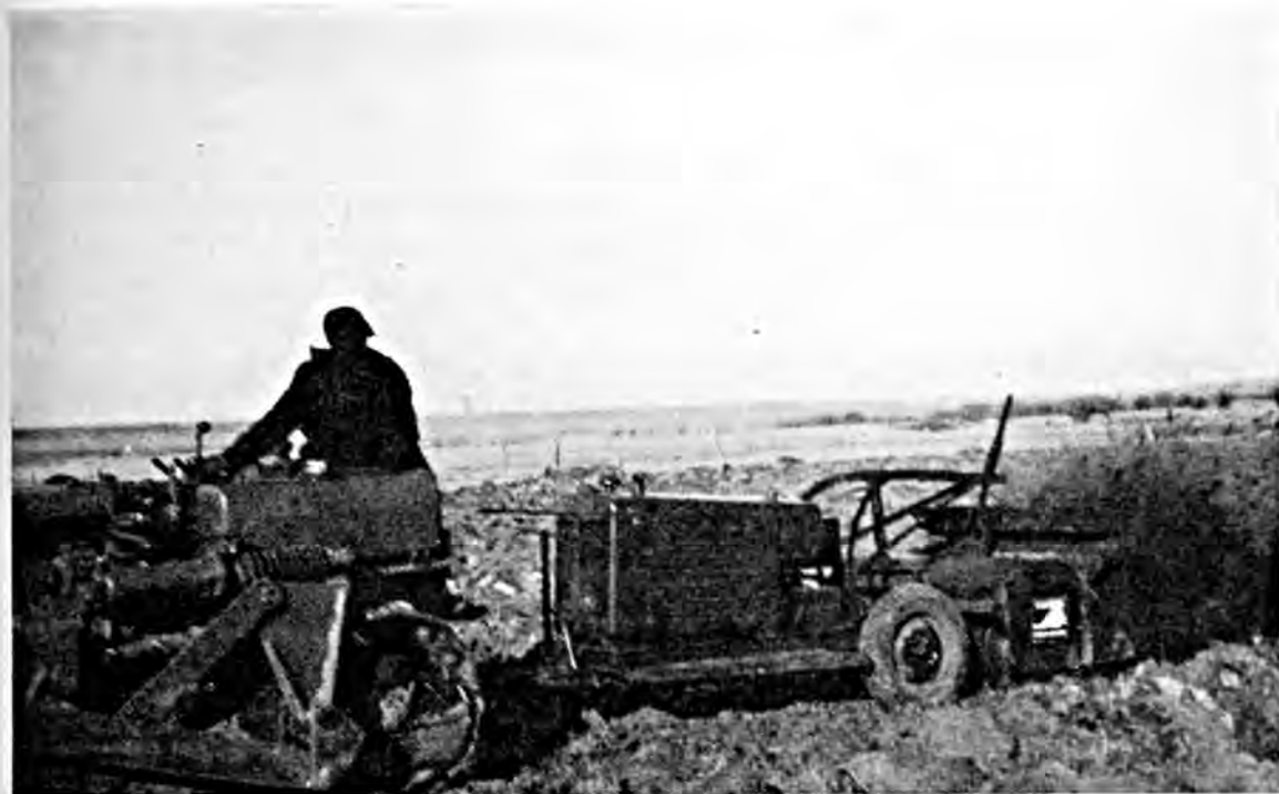
Fig. 2. Side view of tiller shows the mounted gas engine and the pulverized soil being kicked from the revolving hammers.
