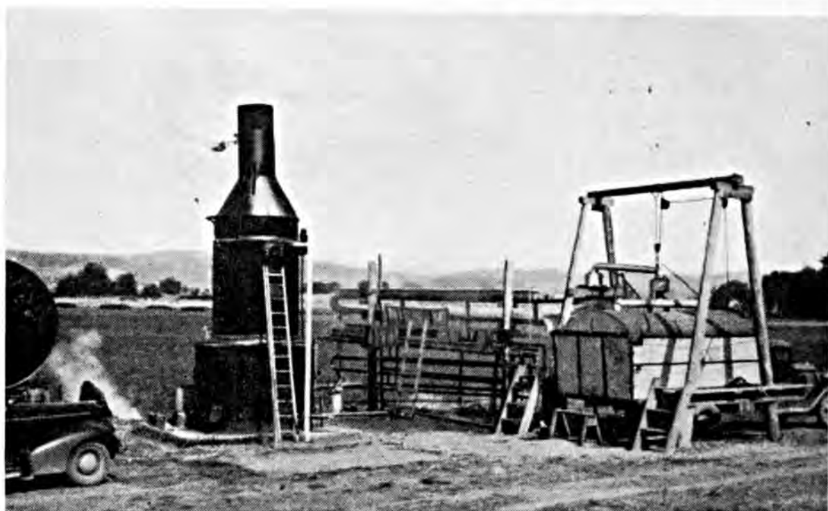
Fig. 4. Boiler; truck with tight bottom and insulated hood for distillation; condenser in rear.
