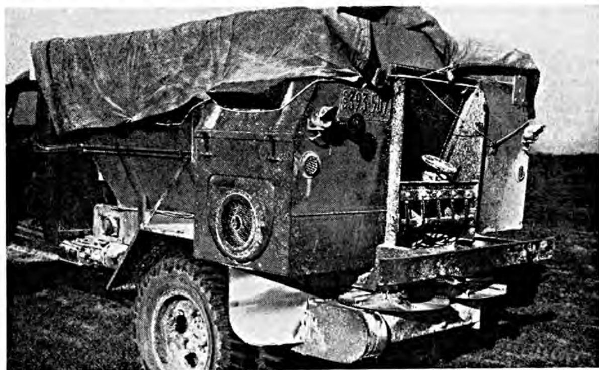
Fig. 2. Close-up of truck. Note enclosed motor at left rear, prongs to break up fertilizer as it falls on fan blades, crank for making adjustments of rate.
