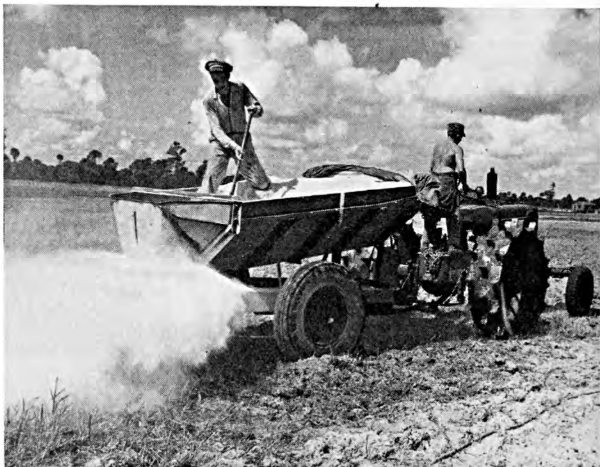
Above: This fertilizer distributor and seeder will spread at the rate of 15 tons per day.
