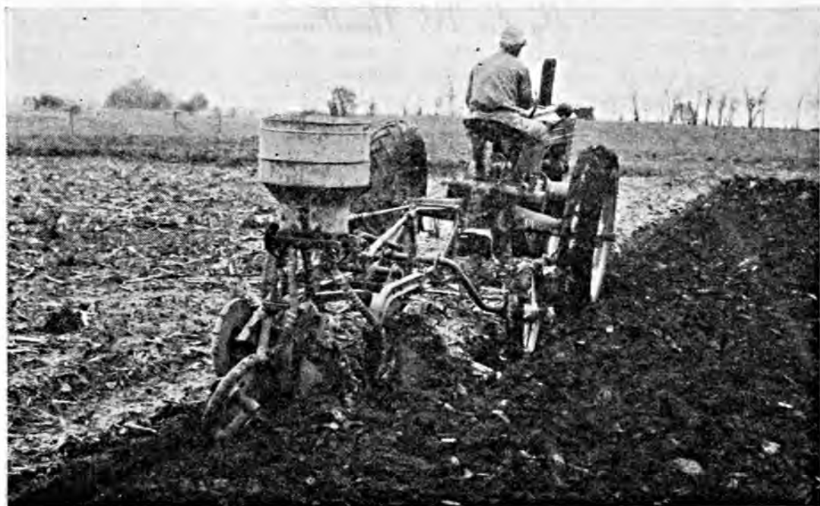
The present method of applying fertilizers deep in the soil is by this attachment over the plow. Growers have found many disadvantages to this method. Carl Thorp solved many of these disadvantages by developing a new machine.
