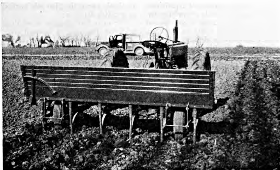
The Thorp deep fertilizing machine in operation. Tubes carry the fertilizer from the large box, capable of holding 500 lbs. of fertilizer, to the base of the field cultivator shovels. The shovels can be regulated to a depth of six inches.
