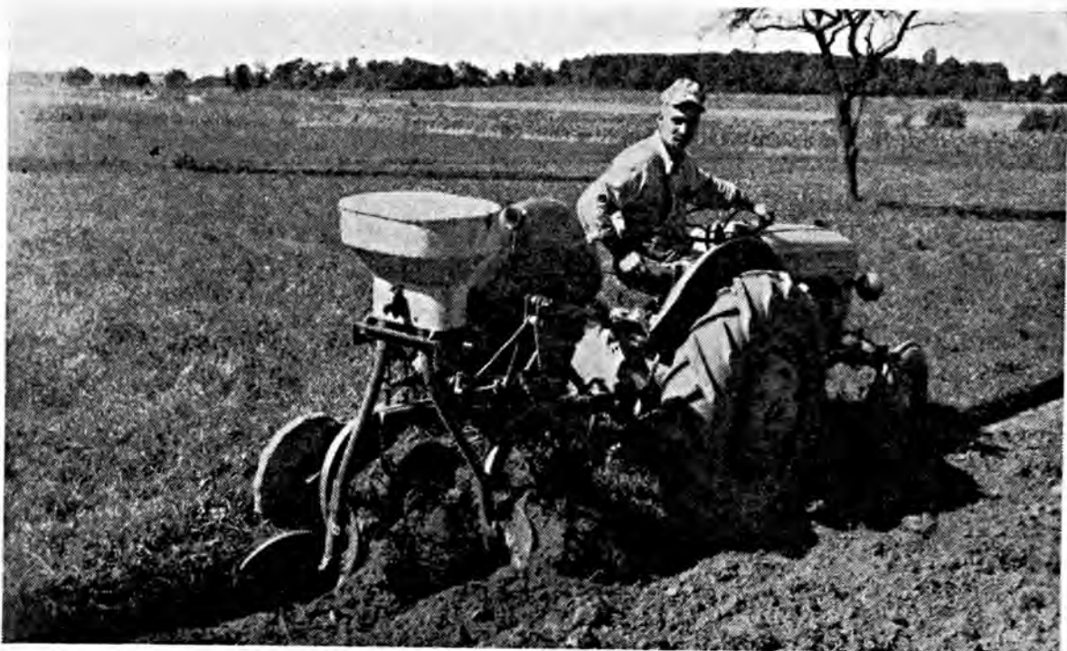
Attachments for the placement of fertilizer on the furrow bottom can be mounted on most any make of plow. Here the equipment is mounted on a Ford Ferguson set of plows.
