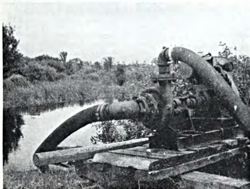
The light, portable pumping outfit used for irrigation at the Dominion Experimental Sub-station, Ste. Clothilde, Quebec. With this outfit water is raised 4\frac{1}{2} feet for 52¢ per acre inch.
