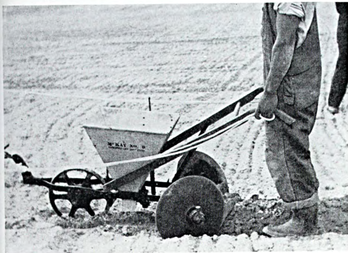
Fig. 5. Combination distributor and bedder used in Method No. 2. This applies the fertilizer, but does not plant the seed.
