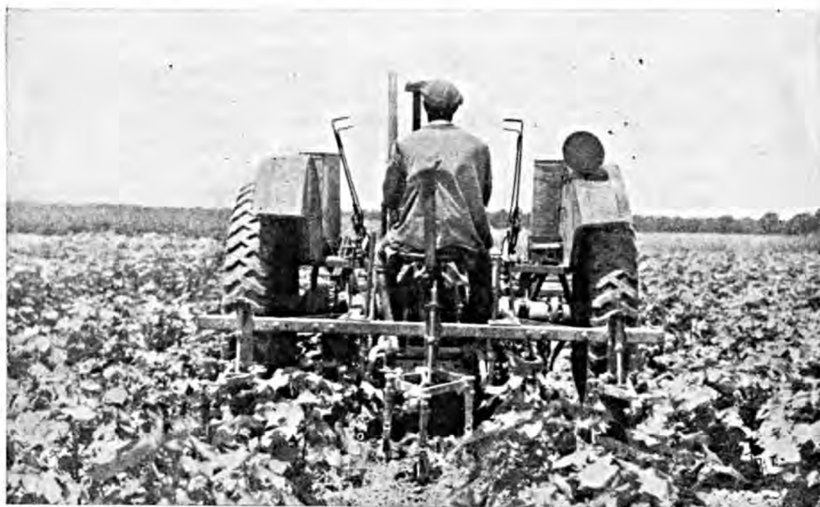
A two-row cultivator and fertilizer distributor, which cultivates the crop and places the fertilizer in bands on the sides of the rows at the desired depth.
