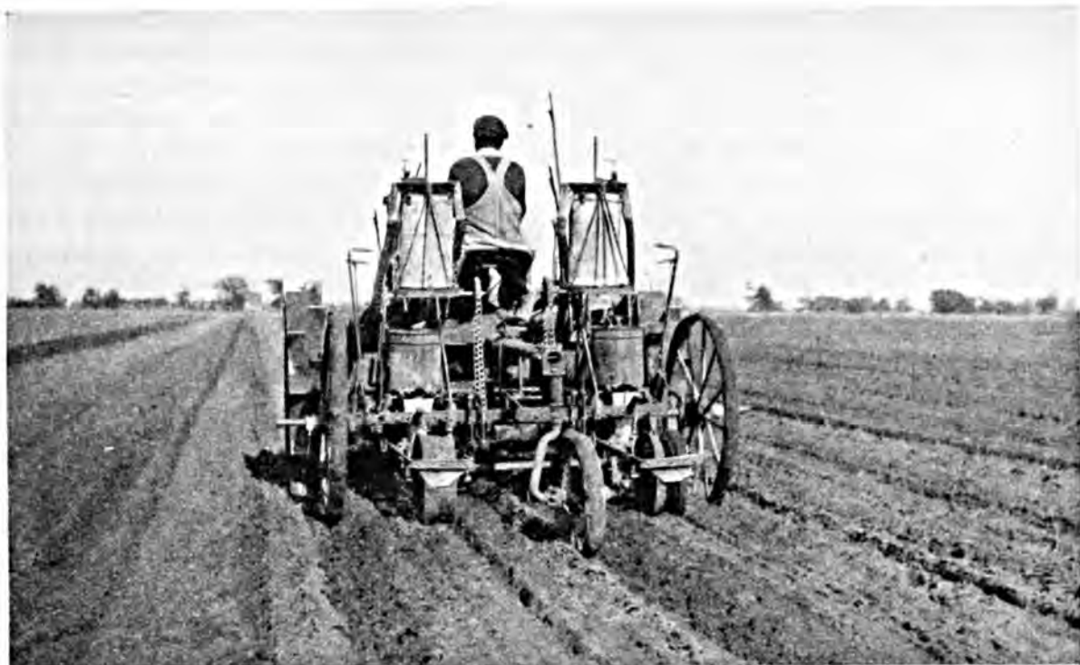
A two-row planter-distributor combination, which applies fertilizer in bands on each side of and slightly below seed band or drill.
