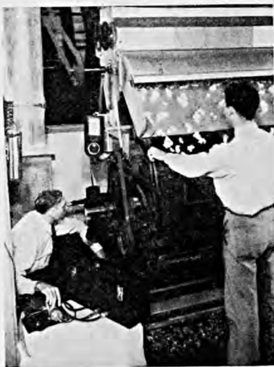
A Stroboscope is used in observing the gin performance.
