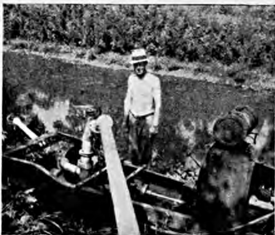
Fig. 1—A centrifugal pump on the Terpstra farm, Hammond, Indiana, was mounted on an automobile chassis and attached directly to the drive shaft, resulting in 20,000 gallons per hour capacity.
