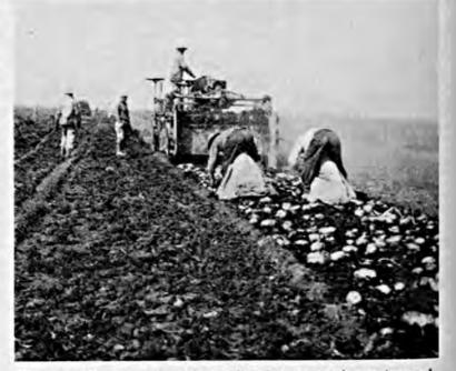
The potato digger used on the Weyl-Zuckerman ranch was invented by Mr. Zuckerman. It digs three rows at a time. Rollers beneath the conveyors leave clean potatoes on well-packed soil.
