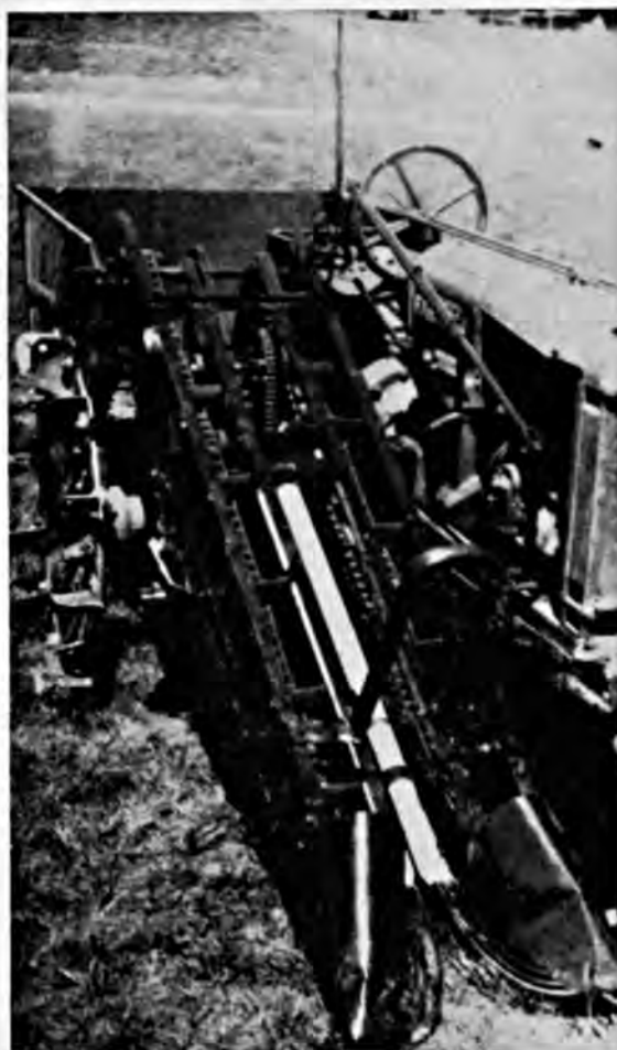
Cotton stripper being developed by the Texas Agricultural Experiment Station. This is the 1931 machine at the beginning of the season.
