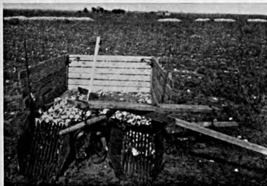
This two-row finger type cotton sled is home-made.
