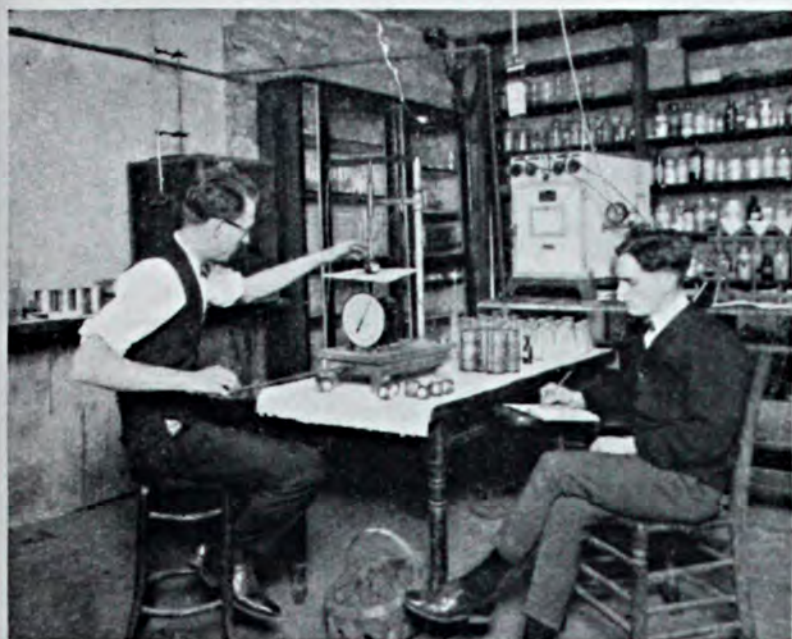
Determining the ripeness of apples in the laboratory by means of a pressure tester.
