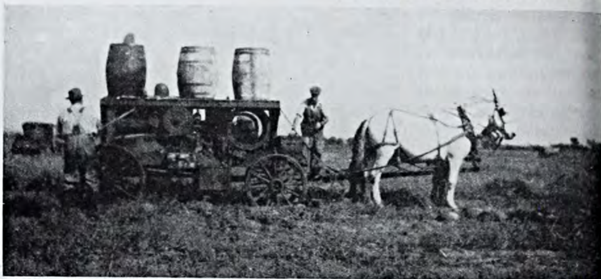
Watermelons from which seeds are to be taken are "threshed" or ground up in a machine such as shown above. The resulting pulp is placed in barrels and allowed to ferment while the seeds go to the bottom after which they are washed and dried.
