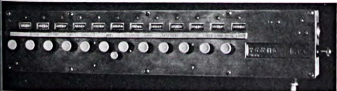
This device is used on automobiles for measuring feet and miles of crops. The operator simply pushes the right crop button.
