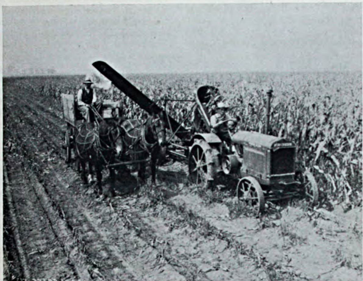
An ensilage harvester converts standing corn to ensilage in one operation. This new method leaves the field clean and delivers high-quality ensilage to the silo.
