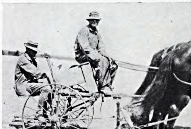
Mr. Traugott made this fertilizer sower from an old discarded sulky cultivator.
