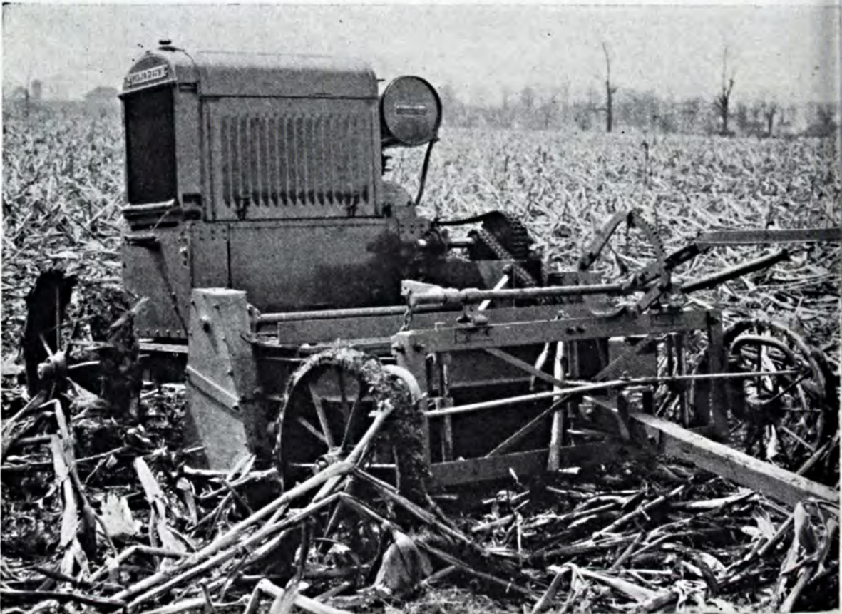
The machine, which was invented by David E. Ross and constructed by the Agricultural Engineering Department of Purdue University, is expected to do much to help keep the corn borer in check.
