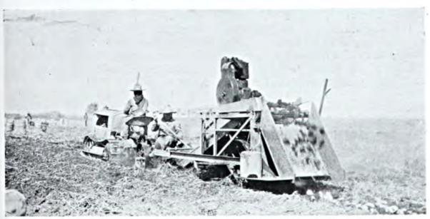
Specially designed potato digger equipped with an auxiliary engine, at work in the delta. This shows the digger without the sacking device.
