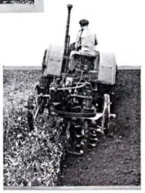
This plow has a rotary attachment for pulverizing the furrow slice.
