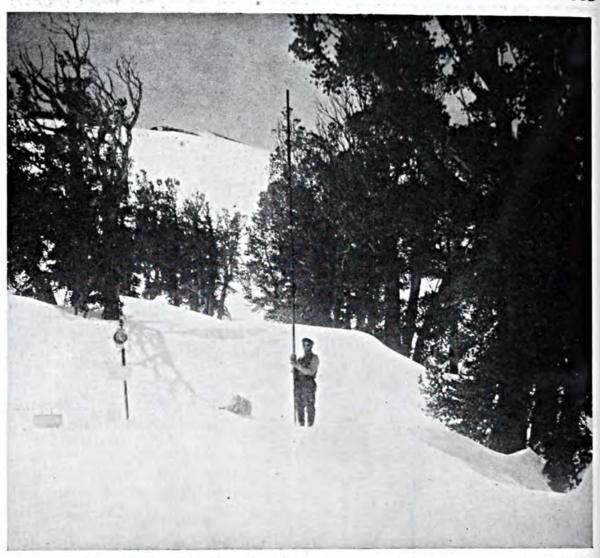
The timber line on Mt. Rose (10,000 feet elevation). The snow is as deep as the sampler is long. Compare the length of the sampler with the height of the observer.
