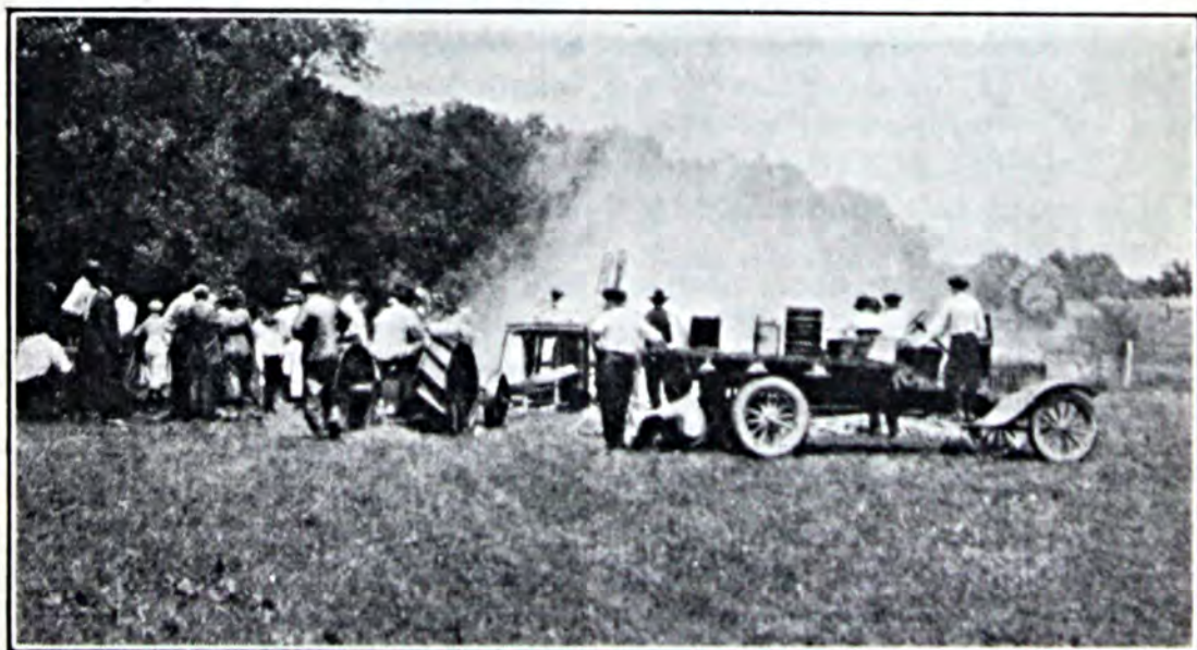
Small limestone crushers were installed in communities not served by railroads. A pulverizing demonstration is being staged in the above photograph
