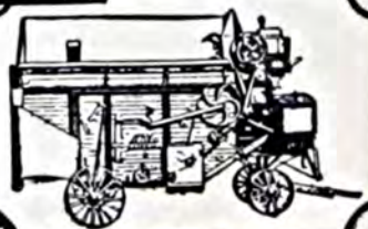
Avery Header Thresher. Harvests and threshes the grain in one opera- tion.
