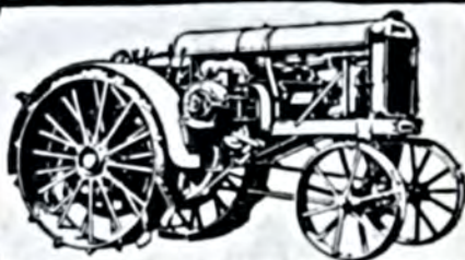
Improved Avery 25-50 H. P. 10-Ton Road- Roller - Tractor. Also built in 45-65 H. P. size
