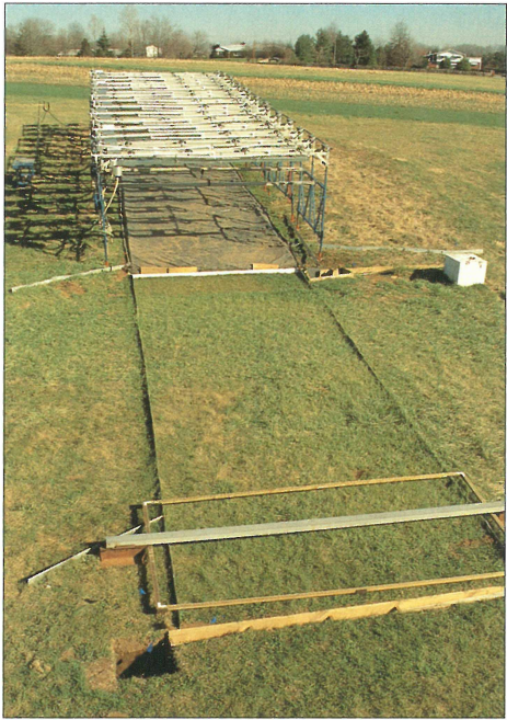
RESEARCH with a rainfall simulator has found significant benefits from use of vegetative filter strips to reduce runoff of potential water contaminants from crop fields.
